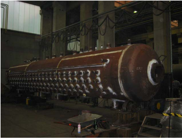
Completed steam drum.
